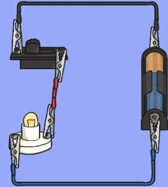
A **circuit with a switch** is not the same as an **incomplete circuit**. In an **incomplete circuit**, the **electrons** are unable to flow at all **whether the switch is on or off**.
